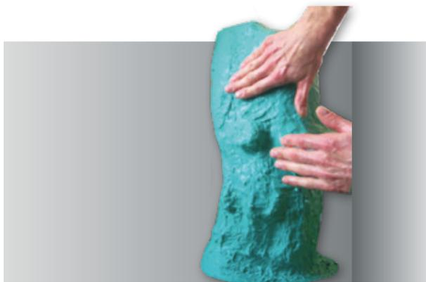
Smoothing the last layer. After finishing the filler layers, it can be smoothed with a mild soap solution to get a homogeneous surface.
