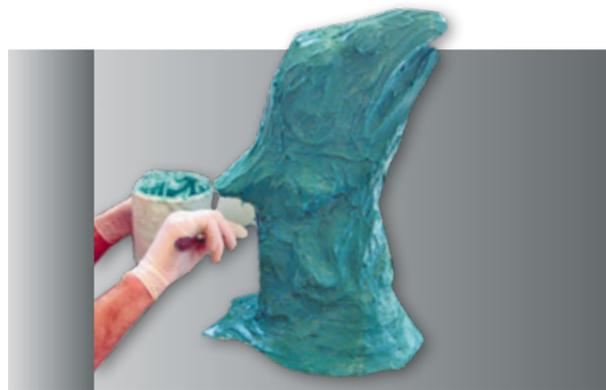
Application of the filler layer(s). To obtain the filled consistency, SILASTIC™ RTV-4250 S is thickened with Thixo Additive RTV-3011. Here a minimum thickness of 5mm is required.
