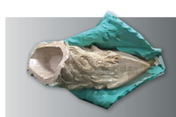
The silicone negative is cut open and removed from the master model. Then the mould is reassembled in reverse order.
