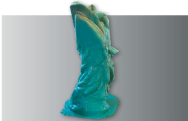
The second layer is also applied thinly after the first layer has gelled. The silicone is now already thickened with Thixo Additive RTV-3011, but still flowable.
