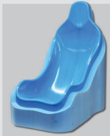
Master model for racing seat tool made of ebalta EP 138
